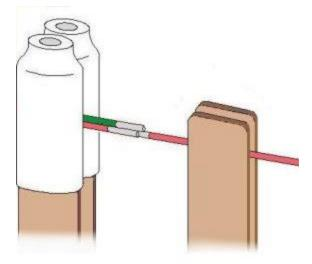
Next, insert the "fish tape" wire through the clip on the right and align it so the end area of its tinned portion is parallel and touching the other two wires. If necessary, use a sharpened toothpick or pointed tweezers to adjust the wires so they are aligned properly.
